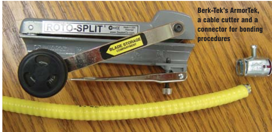
Berk-Tek's ArmorTek™ armored cable
