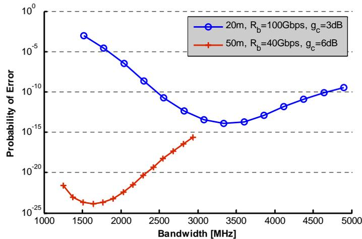
Fig. 5 . Minimization of probability of error through symbol rate optimization for two 40GBASE-T and 100GBASE-T systems.
