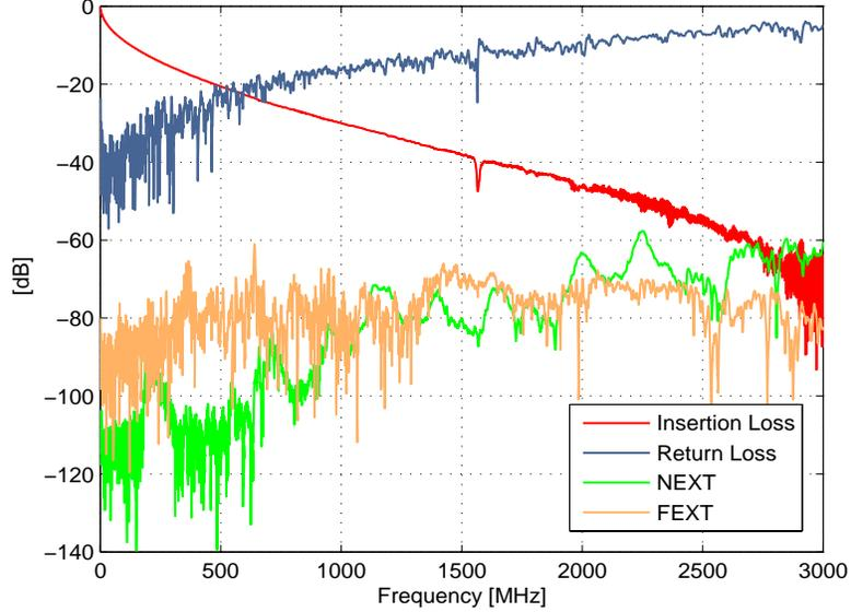
**Fig. 2** Insertion Loss, Return Loss, NEXT and FEXT measurements for 50m CAT-7A.
