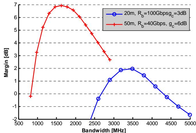
Fig. 6 Maximization of margin for two 40GBASE-T and 100GBASE-T systems.
