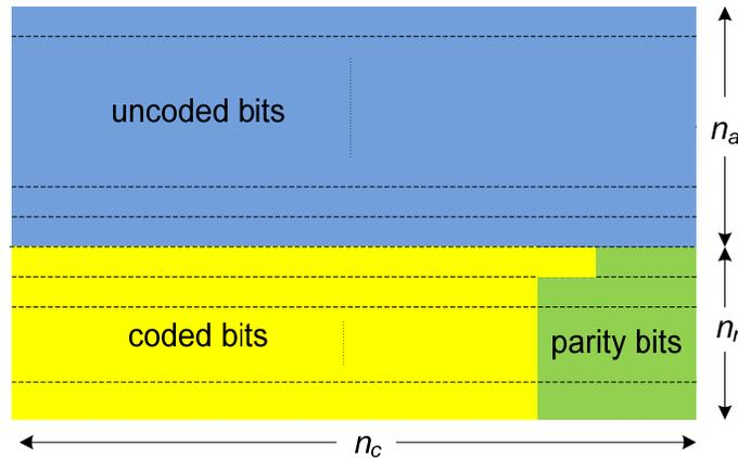
Fig. 8 Construction of block coded modulation.
