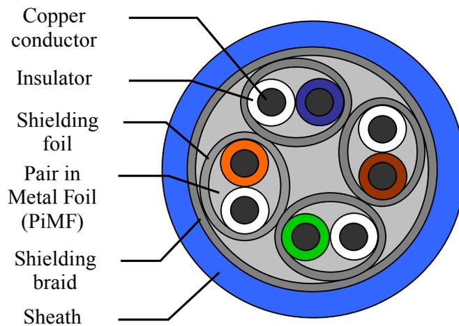
Fig. 1 Cross-section of Category 7 S/FTP cable.
