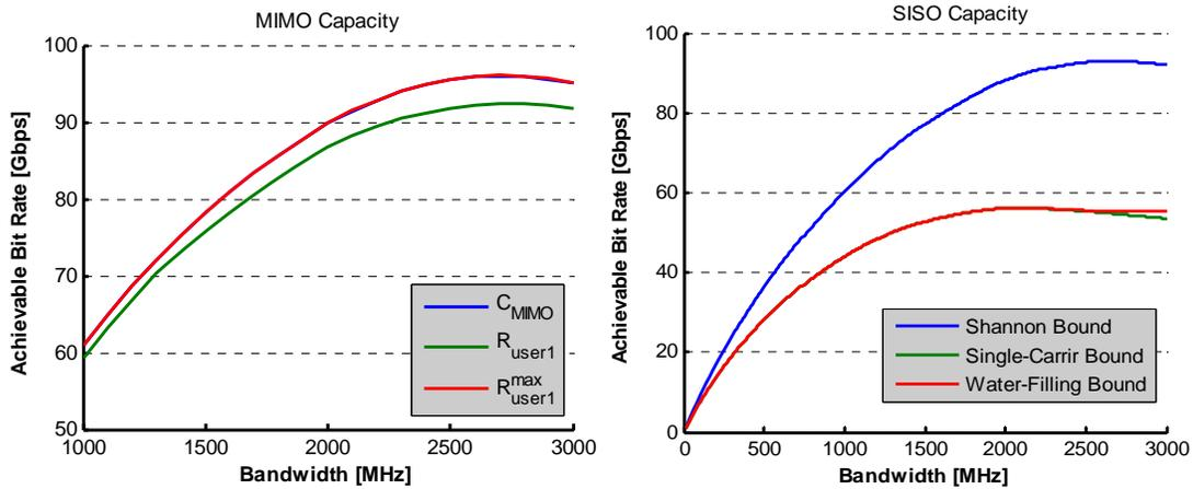
Fig. 4 MIMO capacity and  $R_1$  rate for 50m cable. The SISO Shannon capacity depicted on right is only 3Gbps is less than MIMO capacity.
