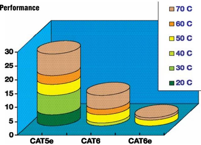
mission distance for a link or channel may be affected. The industry trend to install higher-grade cables, such as Category 6, which utilize larger conductors, minimizes insertion loss while increasing current carrying capacity.
